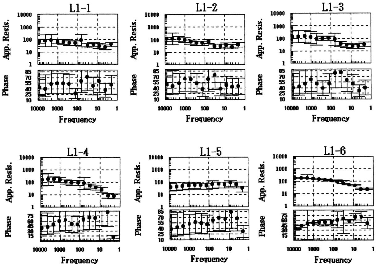
Fig. 3. Graphs of the apparent resistivities (in  $\Omega$  m) and phases (in degrees) with standard errors versus frequency (in Hz) for the sites located along the profile L1.
