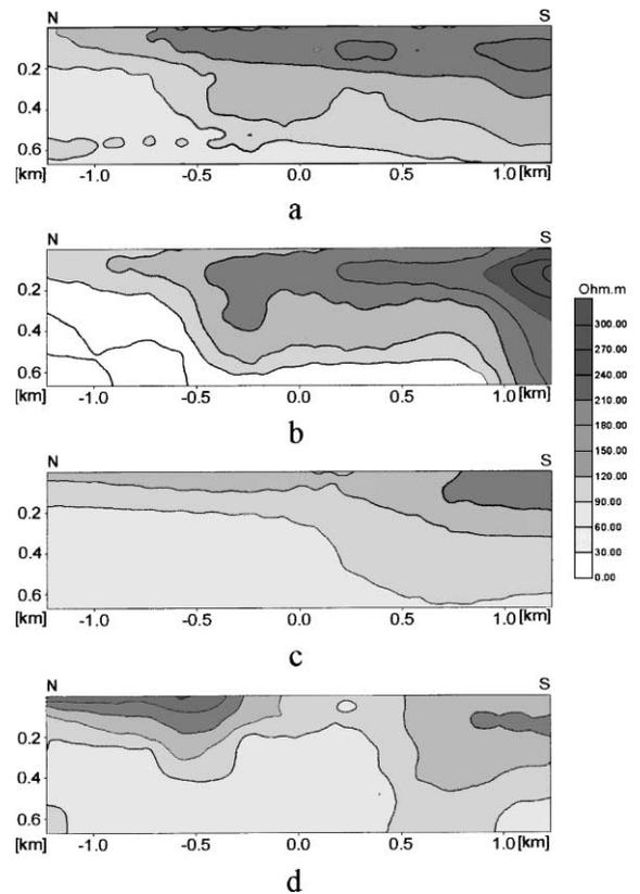
Fig. 9. Apparent resistivity cross-sections beneath profiles L1 (a), L2 (b), L3 (c) and L4 (d) based on syntheses of Bostick transforms.
