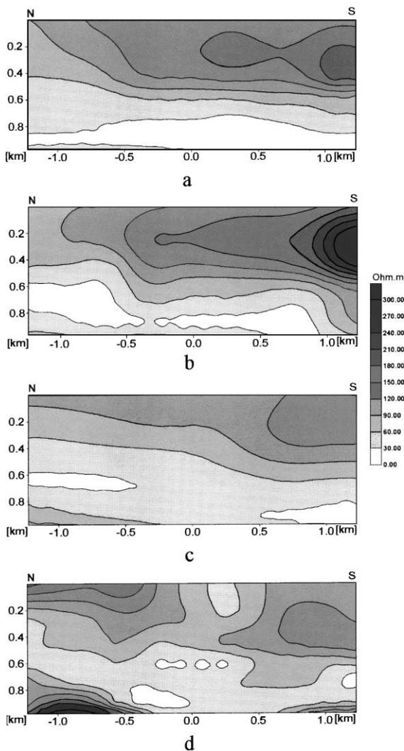
Fig. 10. Resistivity cross-sections beneath profiles L1 (a), L2 (b), L3 (c) and L4 (d) based on 2-D TM Occam's inversion.
