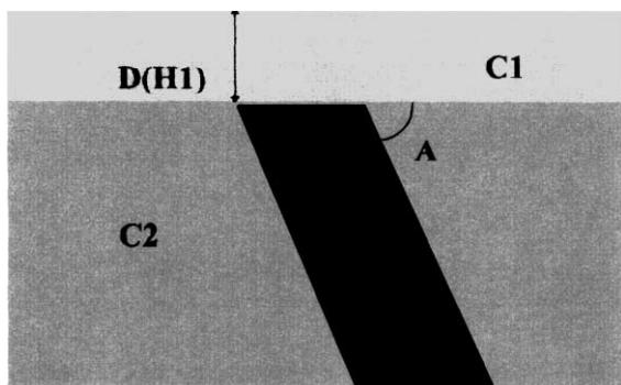
Fig. 11. Vertical cross-section of 3-D geoelectric model used for training ANN:  $C$ ,  $C1$  and  $C2$  — conductivities of the dyke, first and second layer, respectively;  $D$ ,  $W$  and  $A$  — depth, width and dip angle of the dyke, respectively.
