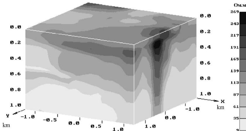
Fig. 7. Volume apparent resistivity image based on 3-D synthesis of Bostick transforms. (Axis  $Ox$  points in the North–South direction).
