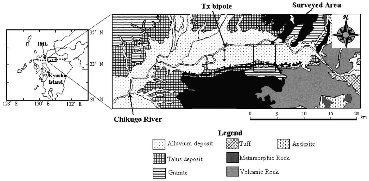
Fig. 1. Geological map of the Minou fault zone. The rectangle outlines the CSAMT survey area. IML—Imari–Matsuyama line.
