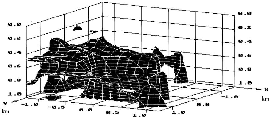
Fig. 8. Apparent resistivity isosurface ( $\rho = 35 \Omega \text{ m}$ ). (Axis  $Ox$  points in the North–South direction).
