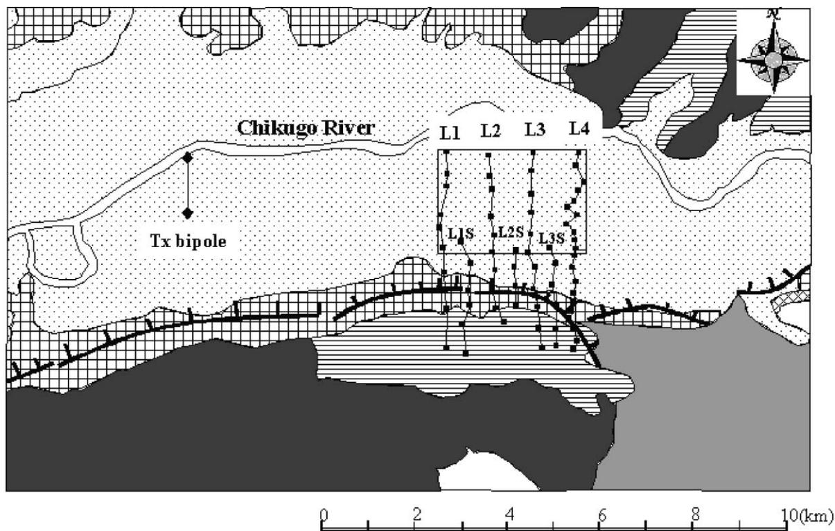
Fig. 2. Site location map (the rectangle defines the northern part of the Minou fault area). Tx—transmitter, L1–L4—survey lines.
