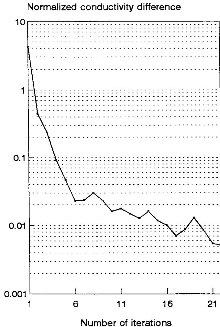
**Figure 2.** Normalized averaged conductivity difference as a function of iteration number for the model shown in Fig. 1.
